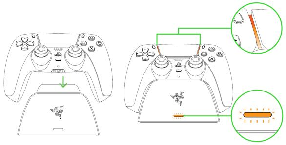
3. Wait for the controller to finish charging. Once fully charged, the light bar on the controller and the charging stand's status indicator will turn off.
